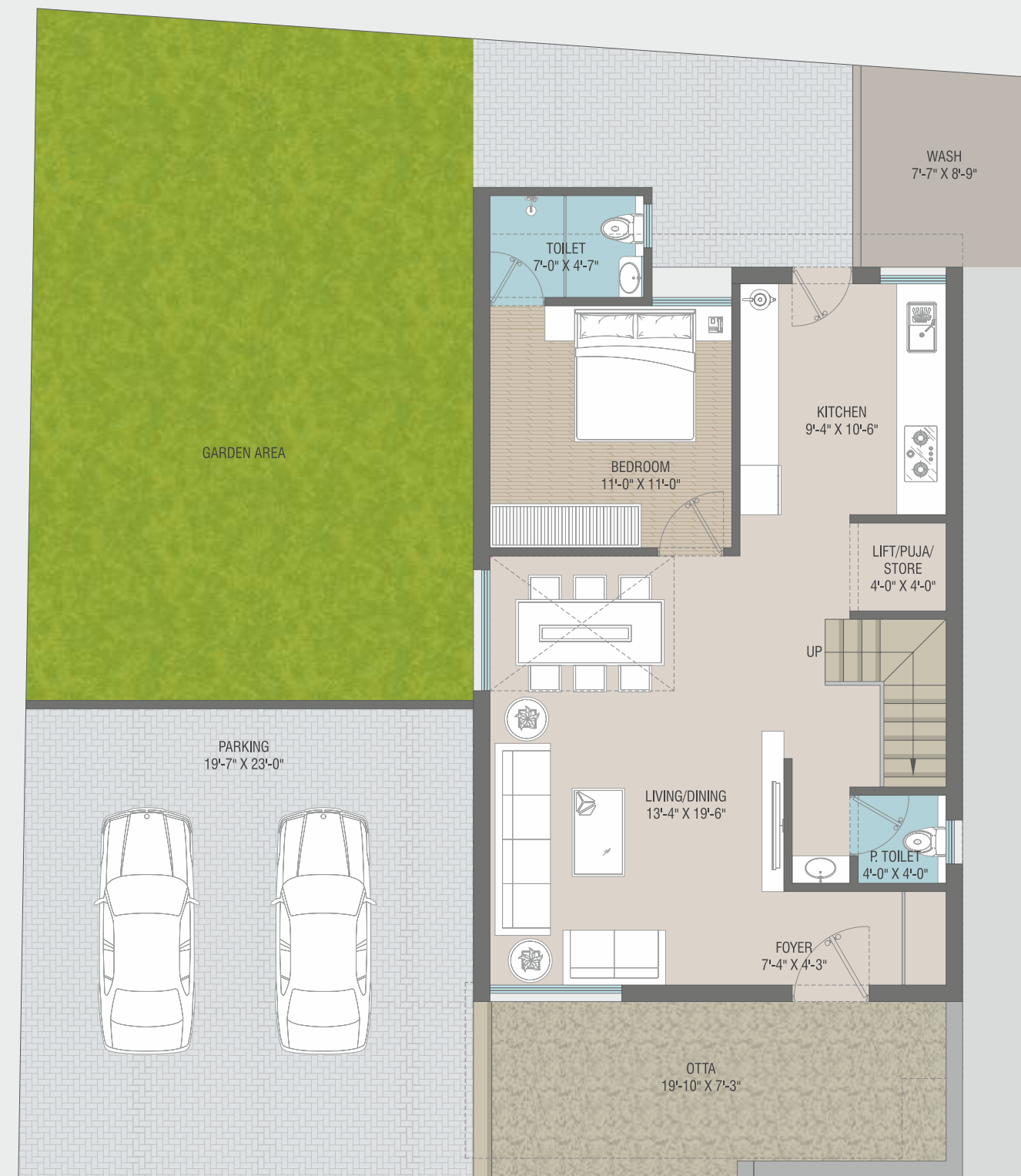
GROUND FLOOR PLAN C.AREA : 674 SQ.FT. BUILTUP : 895 SQ.FT.
