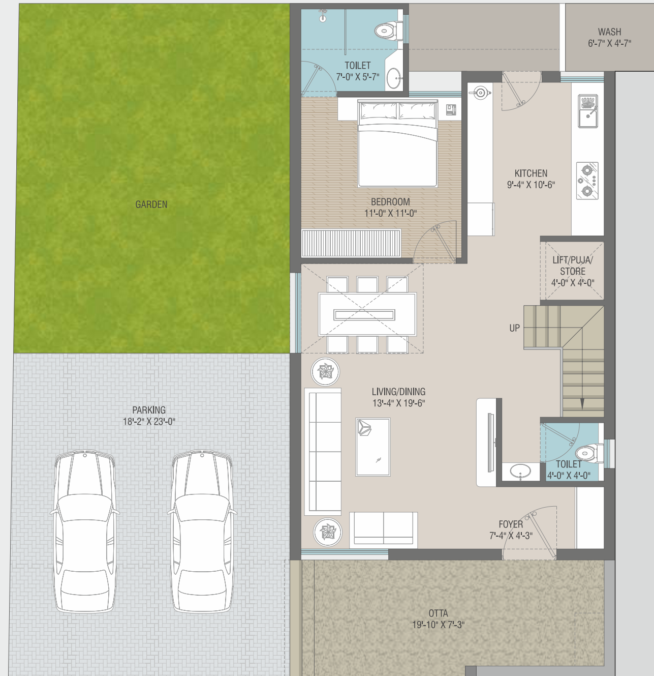
GROUND FLOOR PLAN C.AREA : 681 SQ.FT. BUILTUP : 915 SQ.FT.
